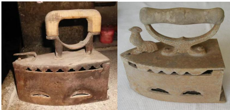
Figure No. (6) The old iron made of cast iron by reheating and putting coal inside it by opening it from the upper moving part.
