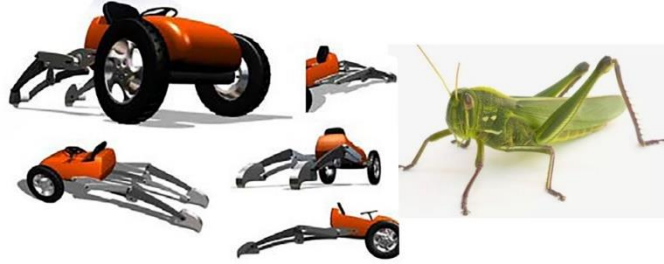
شكل (1) يوضح تصميم جرار زراعي مستوحى من هيكل حشرة الجراد. Jamshid Emami, Mahshid Tashakori And Zahra Tashakorinia, Bionic Design In Industrial Design Education At University Of Tehran, International Conference On Engineering And Product
