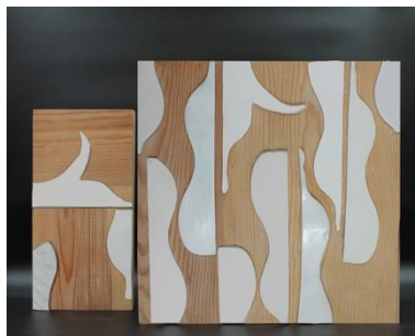
Fig 5. Outcome of the clay experiment: glazed ceramic slab, verity of firing between 06 and 04 electronic kiln.
