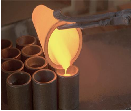
Figure (5) gold casting with lost wax
