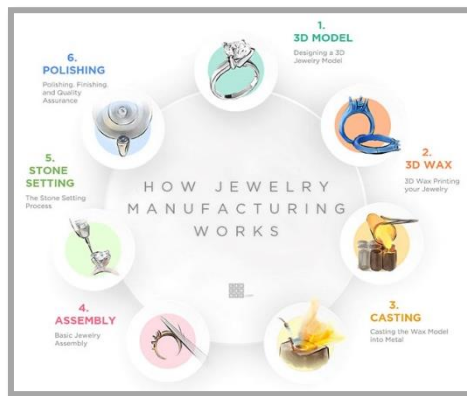
Figure (2) Phases of the formation of metal jewelry
