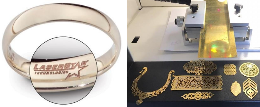
Figure (33) Cutting or engraving jewelry it with a CNC laser machine
